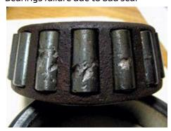
Bearings Failure due to inadequate lubrication
